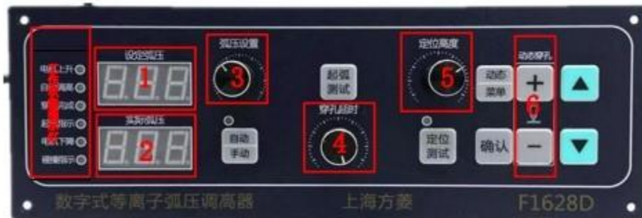
Figure 2. 4 F1628 Series Panel and Key Description
